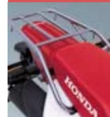
A strong, steel tube rear carrier, designed to hold up to 10kg.
